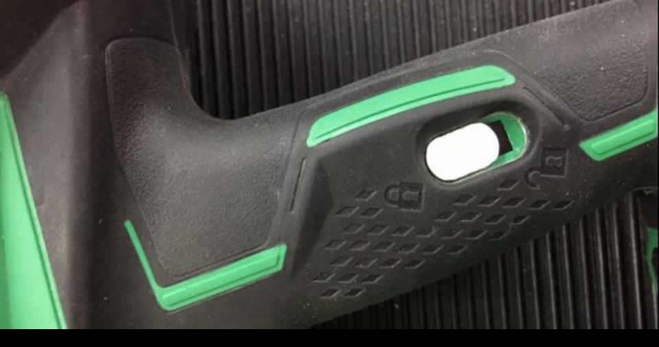
As an extra precaution turn the trigger lock on
