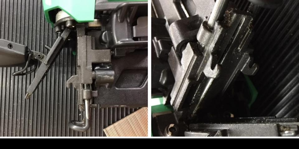
Open up access to top of magazine and clear nail jam
