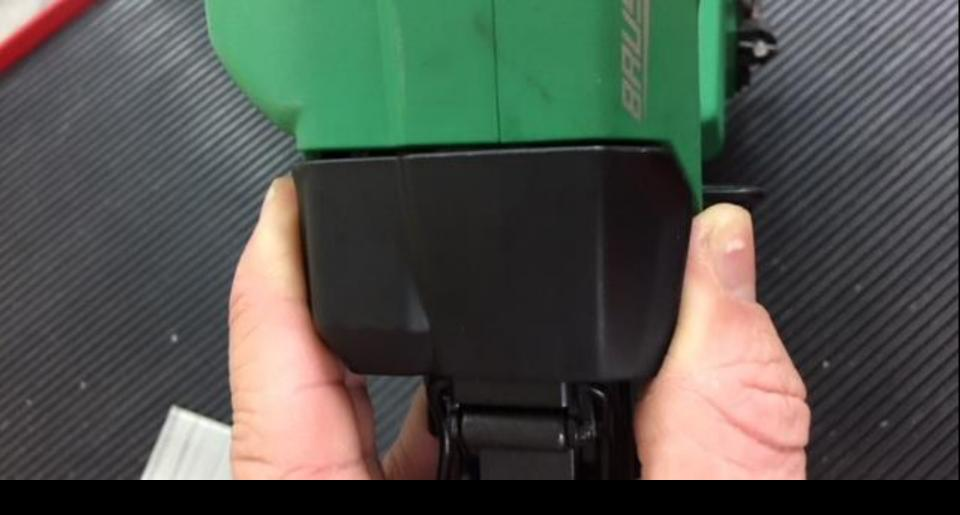
Lift the lock lever for access to the top of the nail magazine
