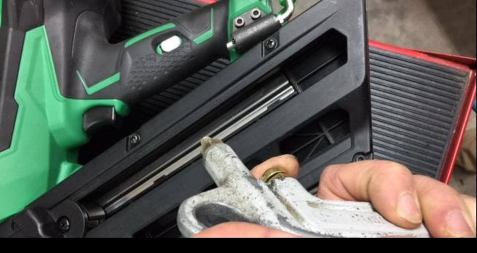
Step 5 - dry off the degreaser, use compressed air (if available or a rag and air dry
