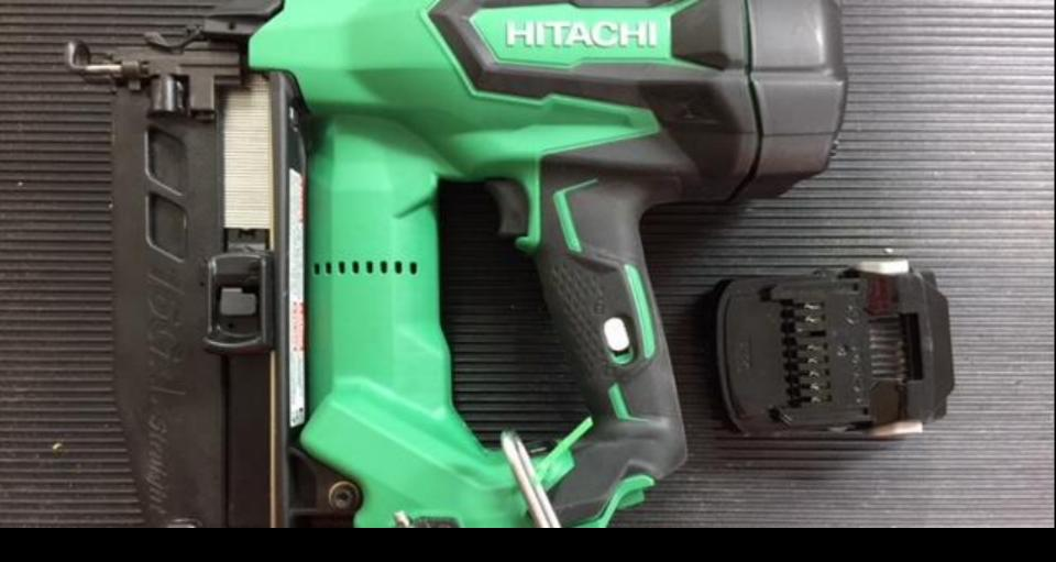
Remove battery from tool to ensure it can not be activated during this process
