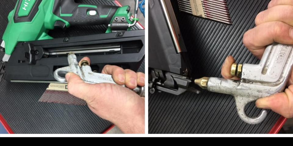
$Step\ 2 \ - \text{If available compressed air is the most simple solution for cleaning the magazine, be as thorough as possible}$
