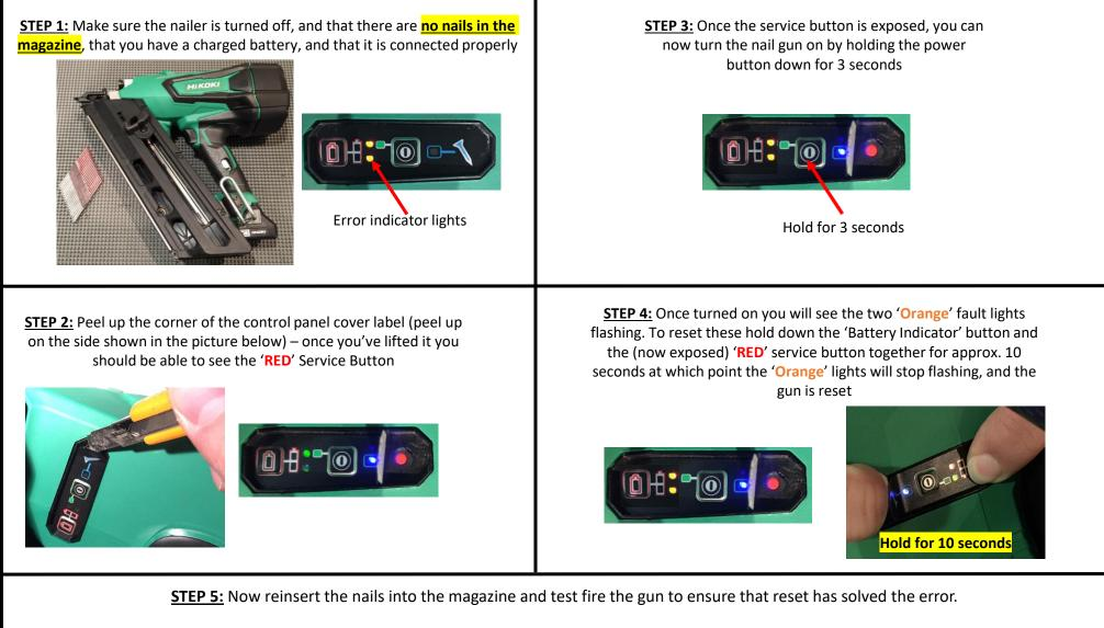
IF THE ORANGE ERROR LIGHTS COME BACK ON AFTER TEST FIRING PLEASE RETURN THE GUN TO A SERVICE AGENT FOR A THOROUGH INSPECTION
